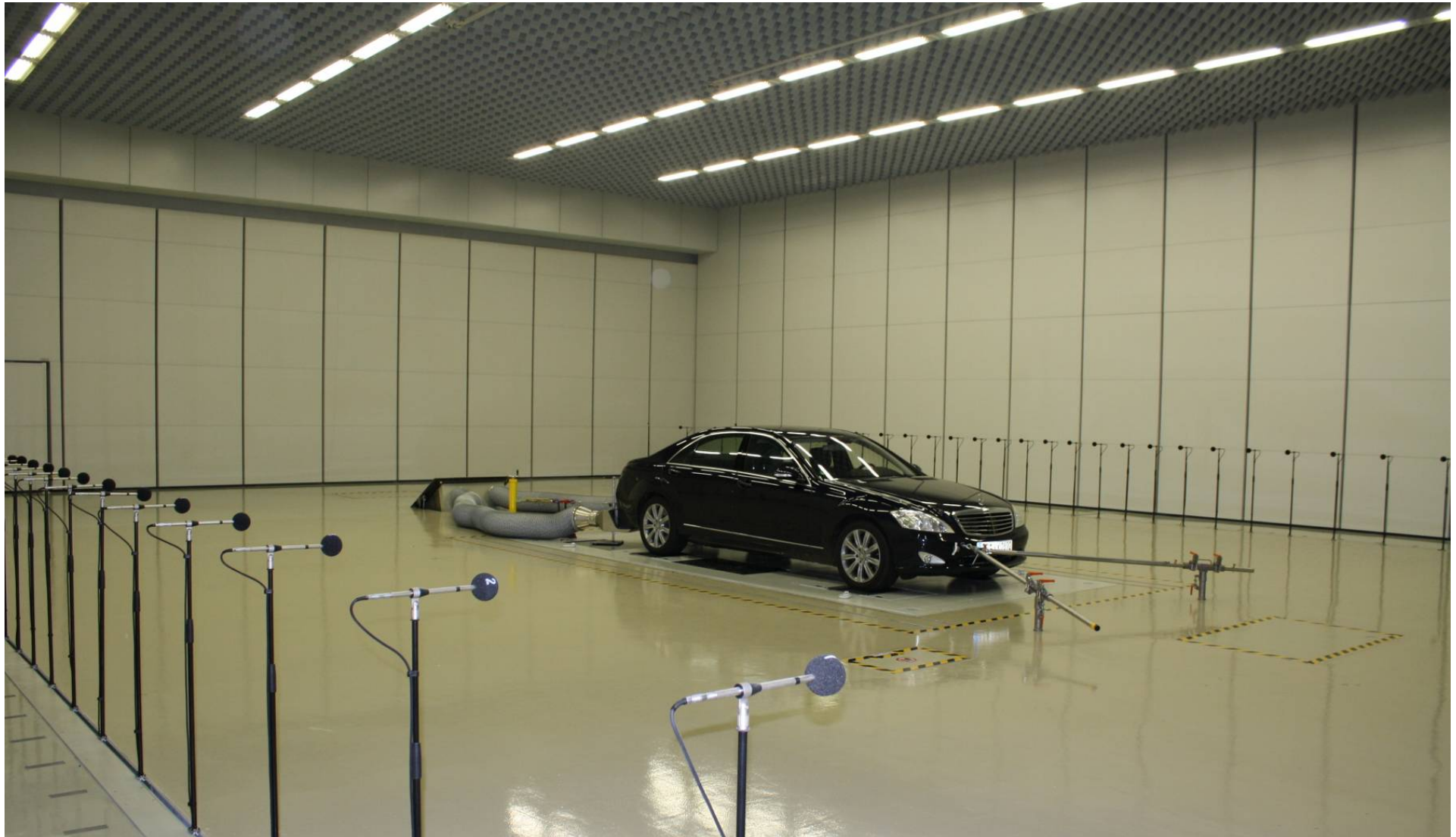
Four-wheel roller test bench in a semi-anechoic room at Fraunhofer IBP.
