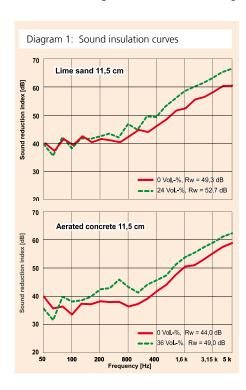
parameters are not equally effective. The maximum moisture-related modification of the weighted sound reduction index in case of aerated concrete is caused for approx. three quarters by the moisture-dependent increase of mass. In case of lime sand this effect causes not even a quarter, since the increase of the sound reduction index essentially occurs due to an increase of the loss factor as a result of the stored water (diagram 3).
