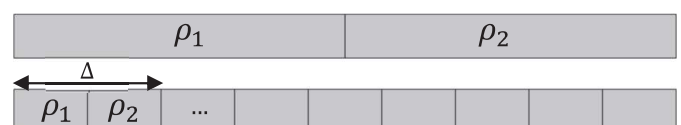
Figure 3: Single (upper) and periodic (lower) impedance jumps, introduced by instant change of the bulk density.
