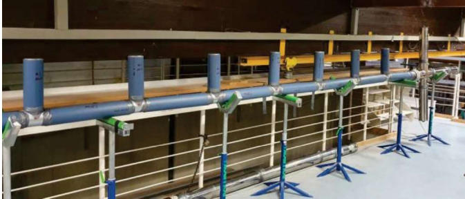
Figure 11: Test setup with seven quarter-wave resonator.
